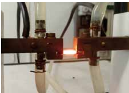
Fracture surface of composites Al 2 O 3 -CNT, carbon nanotubes creates conductive networks (figure on the left). Composite material placed between two electrodes heats up by passing electric current through it (figure on the right).
